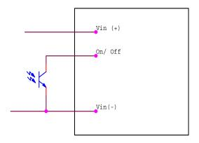
On/Off Circuit for positive or negative logic
